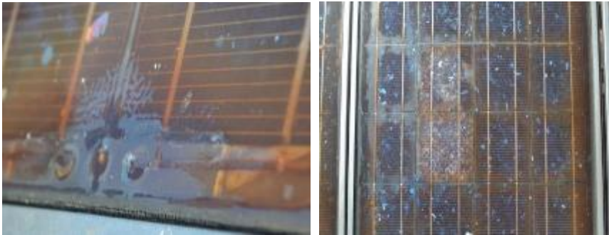
Glass-glass modules with busbar corrosion- Danzhou, China, 15 years
